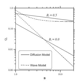
Figure 13. The stability criterion for type-superconductor based on two different two-dimensional heat conduction models. (For  $\dot{\theta}=0.0,~\tau_1=0.0,~\xi=0.0,~\eta=0.0,$  and L=1.0)
