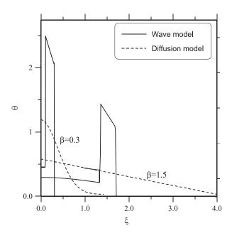
Figure 6. Comparison between temperature profiles obtained based on diffusion model and wave model for type-superconductor. (B=2, f=0.5, Q=0.0, Bi=0.25,  $\theta_{c1}=0.1$ ,  $\dot{\theta}=0.0$ ,  $\tau_1=0.0$ ,  $\eta=0.0$ , and L=0.15)
