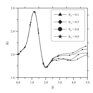
Figure 11. Effect of dimensionless current sharing temperature on type-superconductor thermal stability based on the two-dimensional wave model subjected to stepwise disturbance.  $(B = 2, Q = 0.75, Bi = 0.18, f = 0.5, \dot{\theta} = 0.0, \xi = 0.0, \eta = 0.0, \tau_1 = 0.0$  and L = 1.0)
