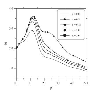
Figure 10. Effect of dimensionless disturbance duration time on type-superconductor thermal stability based on the two-dimensional wave model.  $(B=2, Q=0.0, Bi=0.18, \xi=0.0, \eta=0.0, \text{ and } L=1.0)$
