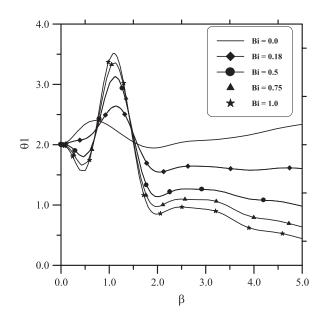
Figure 5. Effect of Biot number on type-superconductor thermal stability based on the two-dimensional wave model subjected. ( $B = 2, f = 0.5, Q = 0.5, \dot{\theta} = 0.0, \xi = 0.0, \eta = 0.0, \tau_1 = 0.0, \text{ and } L = 1.0$ )
